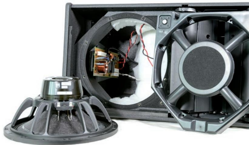
**Torus T1215 with 12" driver**, the phase plug in front and the passive crossover, which contains the components for the high-pass and low-pass filter as well as the small circuit to drive the LED on the front
