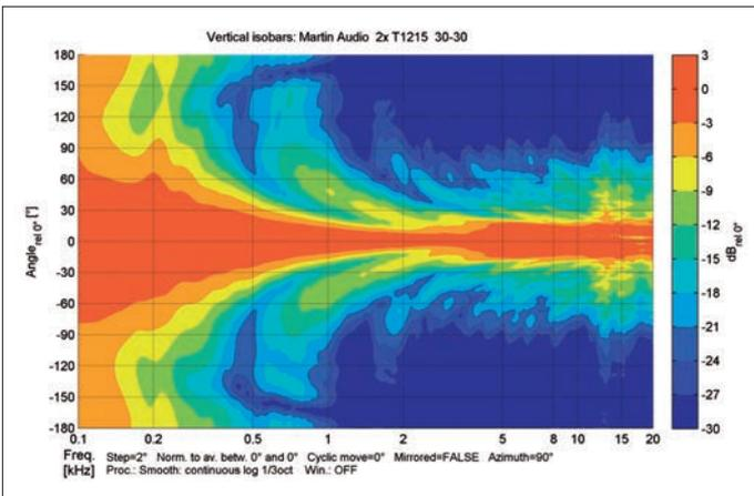
**Vertical isobars** of an array consisting of two T1215s that together cover an angle of 30° (Fig. 11)
