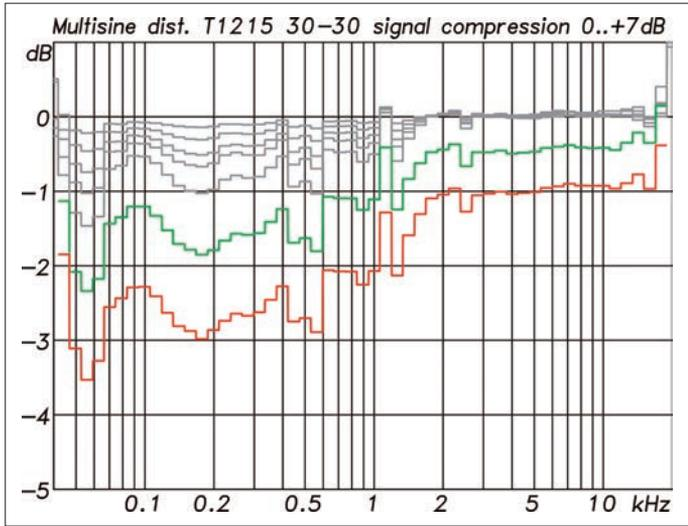
**Power compression** measured with a multitone signal with an EIA-426B spectrum starting at an average level Leq of 113.8 dB. Based on this reference measurement, the input level was increased in steps of 1 dB up to +7 dB. The green curve shows the progression at +6 dB and the red curve at +7 dB. If a broadband power compression of a maximum of 2 dB is permitted, the green curve is the limit. The graph in Fig. 15 was derived from the measurement for the green curve (Fig. 14)
