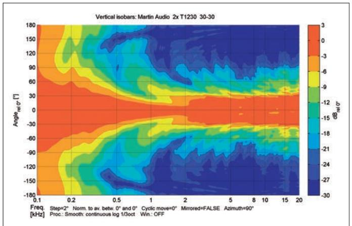
**Vertical isobars** of an array consisting of two T1230s that together perfectly cover an angle of 60° (Fig. 12)
