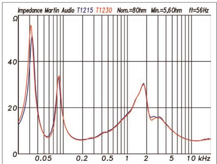
**Impedance curves** of the T1215 (blue) and T1230 (red). The nominal 8-Ω system has an impedance minimum of 5.6 Ω. The bass reflex cabinet's tuning frequency is 56 Hz (Fig. 2)
