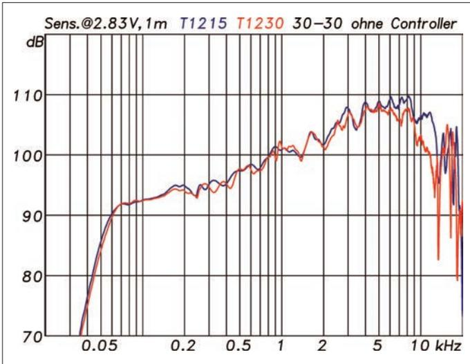
**Frequency response and sensitivity** of the T1215 (blue) and T1230 (red). The internal passive filter is limited to the pure X-Over function. Further filtering is carried out via the controller (Fig. 3)
