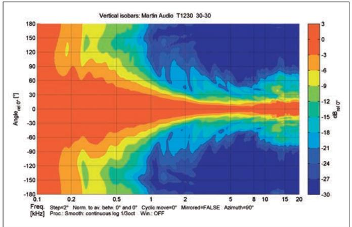
**Vertical isobars** of the T1230 with an opening angle of 30° (Fig. 10)
