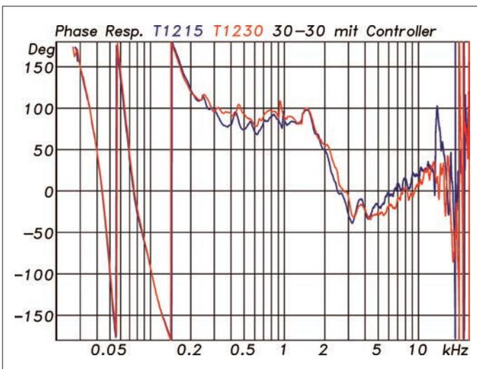
**Phase responses** of the Torus measured as single systems with controller; due to the electrical and acoustic high-pass function, strong phase rotations occur at the lower end of the transmission range (Fig. 5)
