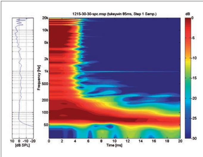
**Spectrogram** of the T1215 with an almost resonance-free oscillation (Fig. 6)
