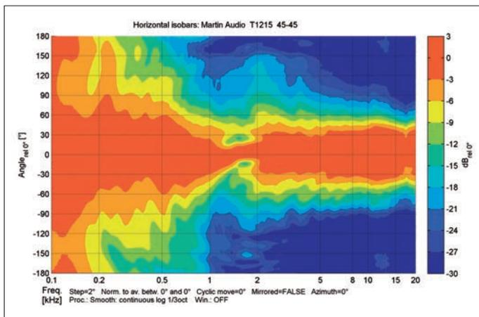
**Horizontal isobars** of the T1215 in the  $\pm 45^\circ$  setting (Fig. 8)
