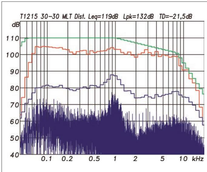
**Intermodulation distortion** of the T1215 with a multitone signal with an EIA-426B spectrum and a 12 dB crest factor for a maximum of 2 dB power compression. In relation to 1 m in the free field, a level of 119 dB as Leq and 132 dB as Lpk were achieved (Fig. 15)
