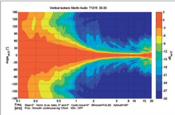
**Vertical isobars** of the T1215 with the narrow 15° opening angle at high frequencies (Fig. 9)
