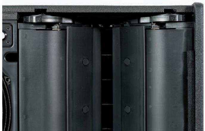
The **opening angle** can be set individually for each side to 30° or 45° degrees via knurled wheels (can also be operated with the grille in place), thus angles of ±30°, ±45° and +45°/-30° as well as +30°/-45° are possible
