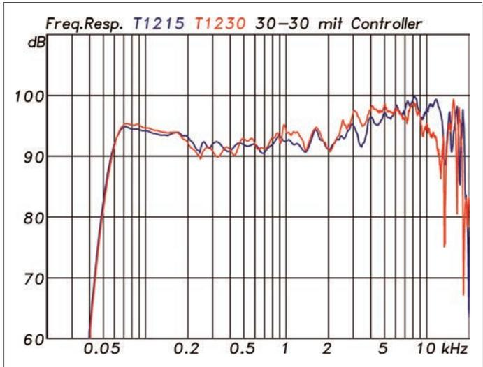
**Frequency responses** of the Torus measured as single systems with controller (Fig. 4)
