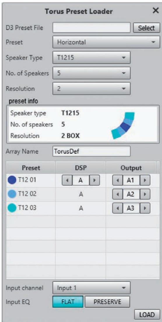
**Pre-set example Vu-NET** for operation of a horizontal array consisting of five T1215s that are controlled via three power amplifier channels (Fig. 16)
