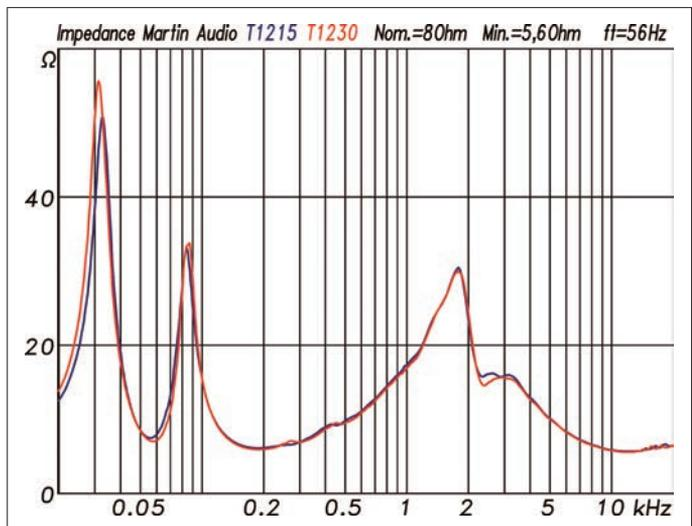
**Impedance curves** of the T1215 (blue) and T1230 (red). The nominal 8-Ω system has an impedance minimum of 5.6 Ω. The bass reflex cabinet's tuning frequency is 56 Hz (Fig. 2)
