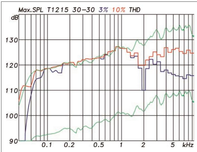
**Maximum level measurement** of the T1215 with sine burst signals for a maximum of 3% THD (blue) and for a maximum of 10% (red) THD. The green curves show the T1215's sensitivity at 1 W at 8 Ω and extrapolated also for 400 W (+26 dB) (Fig. 13)
