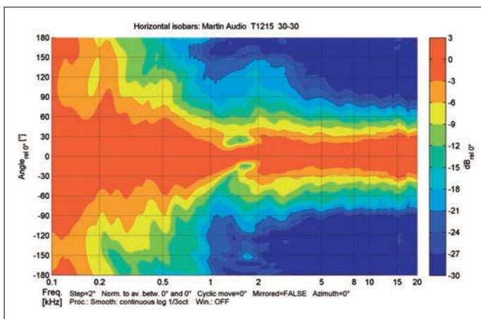
**Horizontal isobars** of the T1215 in the  $\pm 30^\circ$  setting (Fig. 7)
