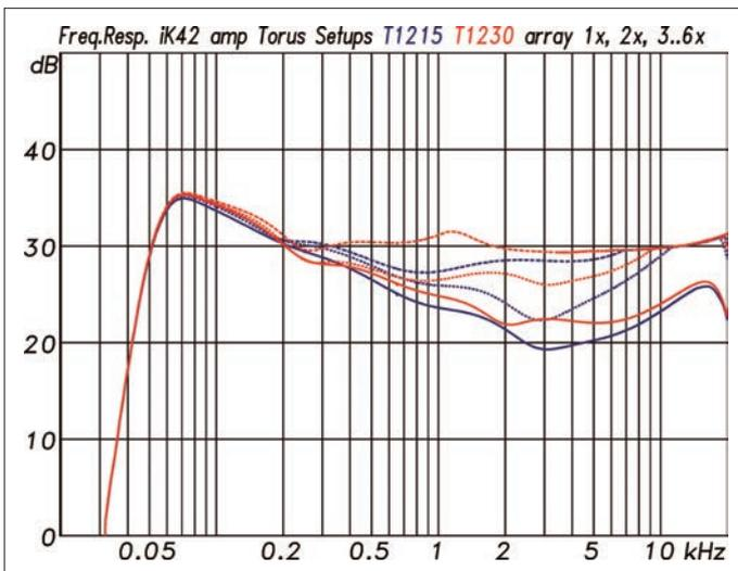
**Frequency responses controller amps iK42** for arrays with one (—), two (---) or three to six (···) Torus units, blue = T1215 and red = T1230 (Fig. 1)
